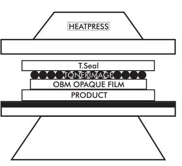
Let cool for a few seconds and remove the T.Seal. Note: T.Seal can be used 100 times and more as long as it is not damaged/teared.
