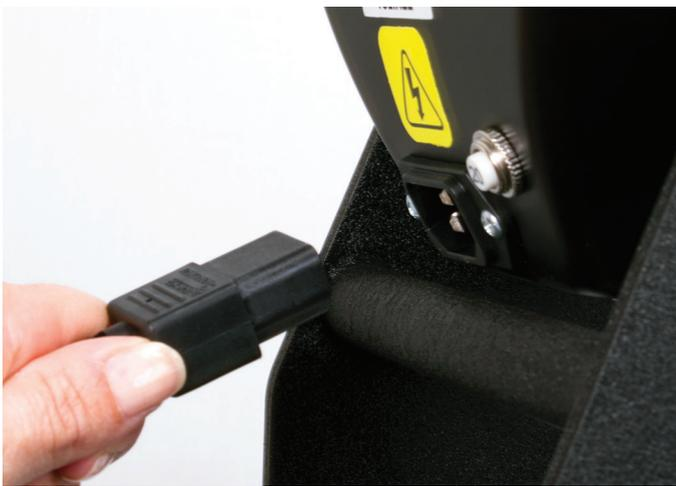
Connect the power cord into a properly grounded electrical outlet with a sufficient amperage rating.
